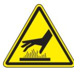
The equipment includes components that reach high temperatures and can cause burns. Hot parts of the equipment must NOT be handled or touched until they have cooled completely.
