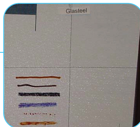
After Stain Cleaning Test
