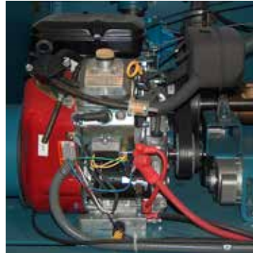
18 HP Briggs & Stratton V-Twin Engine w/positive pressure lubrication system
