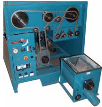
Slideout Airlock System 14" x 14" diameter (35.5cm. x 35.5cm. diameter) 4" (10cm.) Outlet
