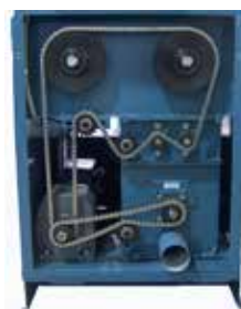
Clear Acrylic Safety Guard Allows for Inspection
