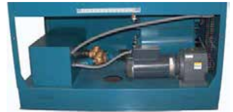
2 HP Direct Drive Motor/Reducer w/overload protection of transformer
