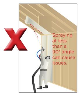
**DON'T** spray at an angle because it may negatively affect the adhesion of the foam.
