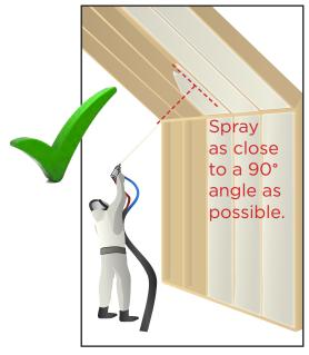
**DO** spray perpendicular to the deck, from the bottom to the top.
