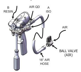
6. Turn on air and open ball valve (air). Air should now flow through the mix tip with gun not triggered.
